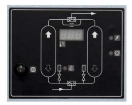
The electronic Pressure Dew Point control (CD) extends the drying phase of the dryer's cycle. It is done by measuring PDP of compressed air on the dryer outlet and only switching the columns when desiccant in the active tower is saturated. The regeneration part of the cycle stays fixed.
